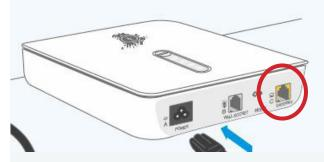
3. Run the supplied white network cable from the blue WAN port on the TP-Link Router to the wall socket or the Lan1 socket on the nbn NCD.
