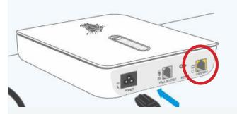
3. Run the supplied white network cable from the blue WAN port on the TP-Link Router to the wall socket or the Lan1 socket on the nbn NCD.
