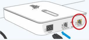
3. Run the supplied yellow network cable from the blue WAN port on the TP-Link Router to the wall socket or the Lan1 socket on the nbn NCD.
